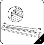
7. Release cover screw, then open the base unit cover
