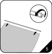
5. Open the snap bar then insert the top edge of the graphic.
