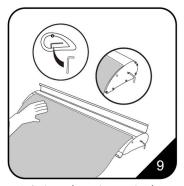
Activate the spring tension by removing the Allen Key. Pull the Allen Key while holding on the the attached graphic. Save the key in the side cover.
