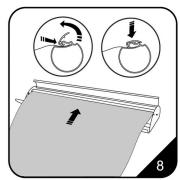
8. Open the roller's lid, slide the bottom edge of the graphic under the lid. Close the roller's lip to secure the graphic.
