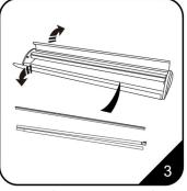
3. Open base unit's cover, pick out the telescopic pole and snap bar.
